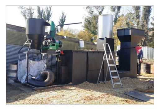
Figure 4: A biochar retort from New England Biochar. Photos courtesy of Wilson Biochar Associates.
