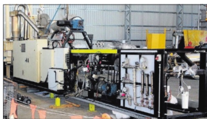
Pyro Ag is an organic by-product collected from the manufacture of Bio-Char in a Continual Biomass Converter.
